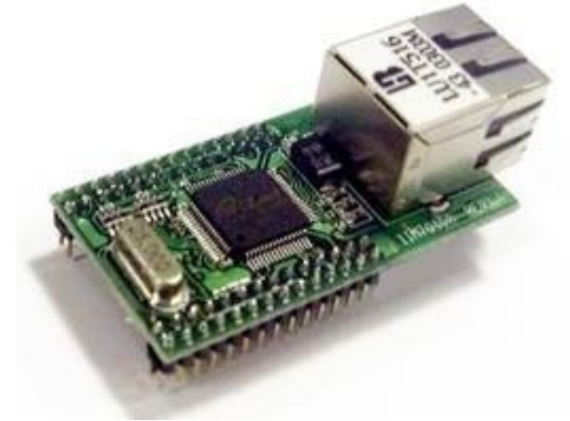
Fig: An example of a COTS product for TCP/IP plug-in from WIZnet (WIZnet NM7010A Plug in Module)
